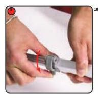
Push down on the lever to lock the rail into place
