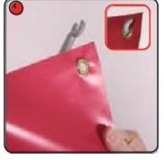
Attach the top graphic eyelets to the support arm hooks.
